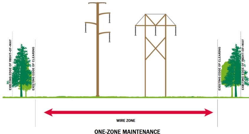
*The diagram illustrates a typical right of way condition. This work is occurring within the existing edge of clearing. Your neighborhood may have a different configuration of transmission structures.*
