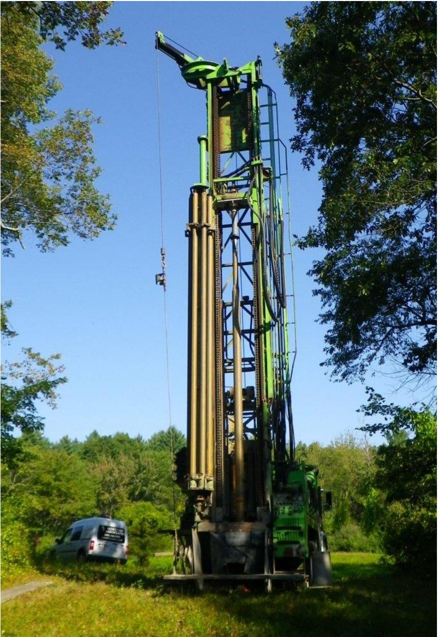
Typical Bedrock Well Drilling Rig
