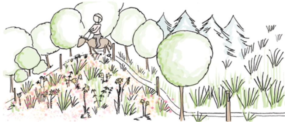
FIGURE 20.1: Blazed posts line the meadow trail to help establish new trail patterns while the meadow gets established. The meadow trail stays close to the meadow edge, and provides a climbing-turn to prevent cross-contour erosion.
